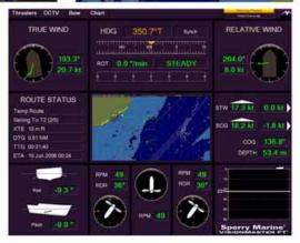
The VisionMaster CID shows critical navigation sensor data in a clear, easy-toread format, and can be integrated with VisionMaster options such as CCTV.
